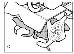
Figure 9: "A" - all four tine gangs in standard position; "B" - two outer gangs removed for narrow tilling; "C" - the two inner gangs have been swapped for stony tilling conditions.
